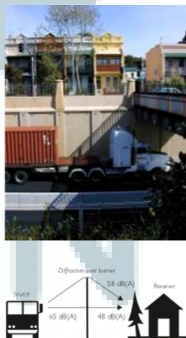
Figure 3. The Acoustic Effectiveness of a Barrier (Source: RTA, page 17, 2001)
