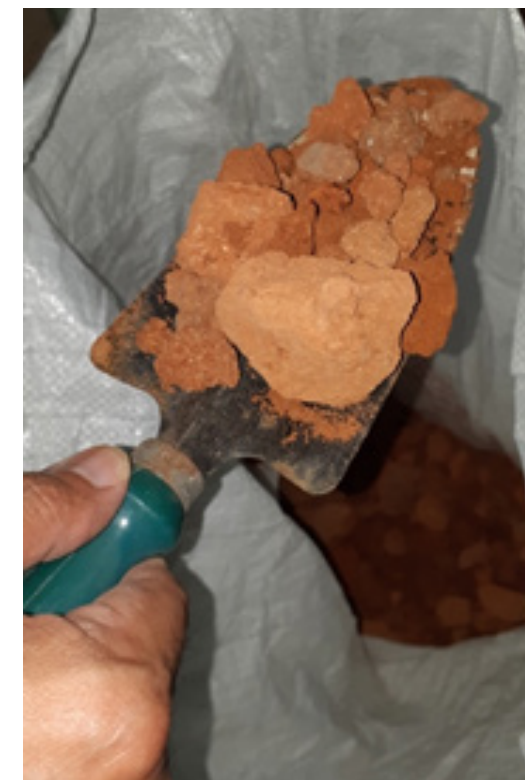
Figure 8. Insert coarse aggregate into the research box (source: processed by researchers)
