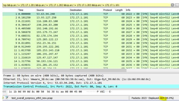
Figure 10. Captured SYN Flood Diverted to SYN Proxy
