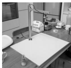
Fig. 2. Image Scanner Using Tower Platform and Webcam Installed on The Top
