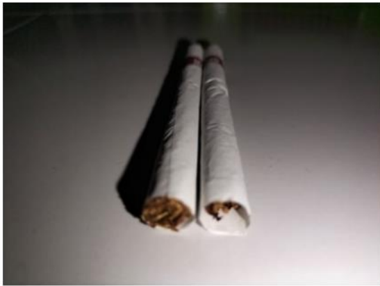
Figure 9. Normal and Artificially Loose-End Defective Cigarette
