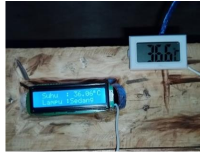
Fig. 12. Comparison results of temperature sensors with thermometer
