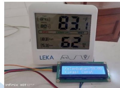
Fig. 13. Comparison results of humidity sensors with hygrometer
