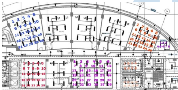
Fig. 5. Tower D's Classes, Laboratories, Architecture Studios, Toilets, and Storage Measurement Points
