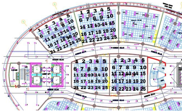
Fig. 4. Tower C Seventh Floor for Laboratories Measurement Points
