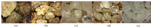
Fig. 3. Image Dataset: (a) Cipongkor River Sand, (b) Sand Citarum River, (c) Cream Silica Sand, (d) Brown Silica Sand, (e) White Silica Sand
