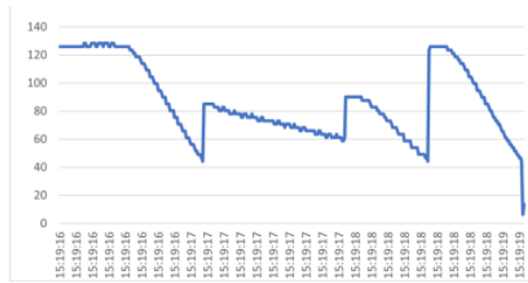
Fig. 13. PWM response of the robot on 3-point coordinates of the untextured path
