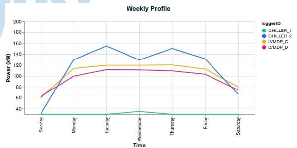
Fig. 10. Weekly profile of power consumption Chiller 1 and 2 and LVMDP of buildings C and D
