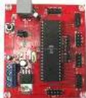
Gambar 4. DT-AVR Low Cost Micro System.
