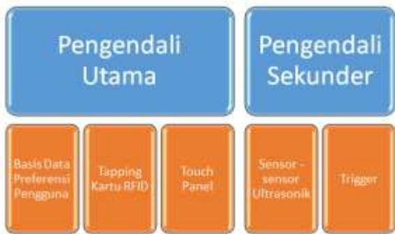
Gambar 1. Blok Diagram Sistem Piano Stairs
