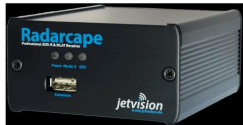
Gambar 7. ADS-B receiver Radarcape
