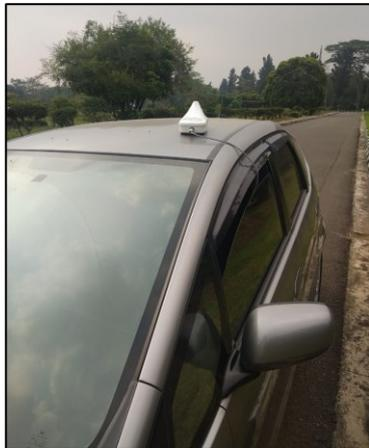
Gambar 11. ADS-B Transmitter dipasang diatas Mobil
