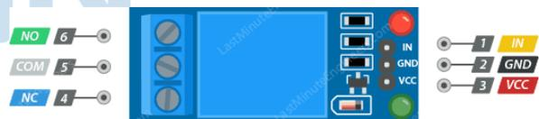
Gambar 3. *Pinout single relay* 5V
