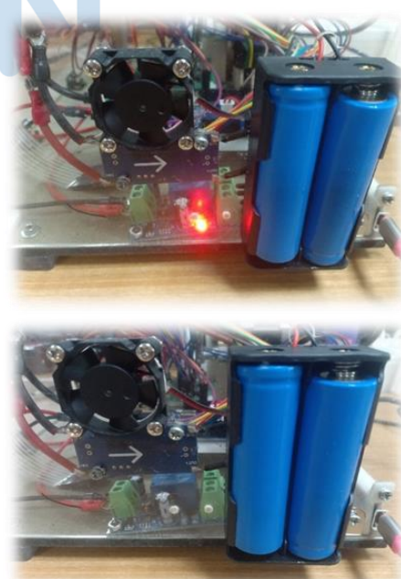
Fig. 9. Above: PMS state when using AC power adapter. Below: PMS state when using battery DC power
