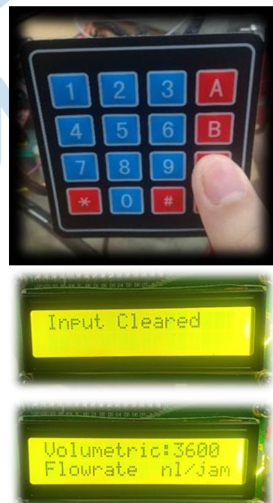
Fig. 6. Top: Process of pressing keys on the keypad. Middle: Pressing the C key, the input is deleted and then ready to accept the new entry. Bottom: Receipt screen enters volumetric flowrate and enter numeric data
