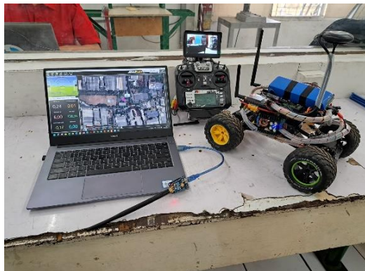
Fig. 2. (a) Rover Schematic, (b) Rover with Ardupilot controller
