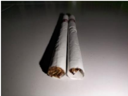
Figure 9. Normal and Artificially Loose-End Defective Cigarette
