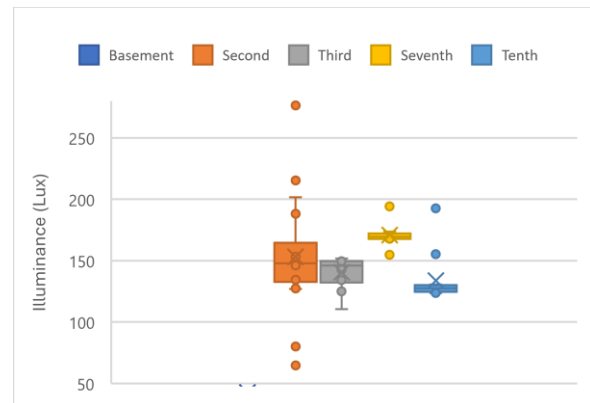
Fig. 11. Box Whisker Plot for C Tower Illuminance Calculation Results
