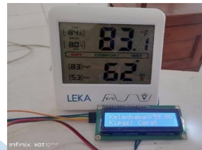
Fig. 13. Comparison results of humidity sensors with hygrometer
