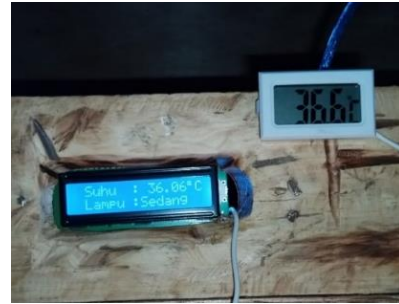
Fig. 12. Comparison results of temperature sensors with thermometer
