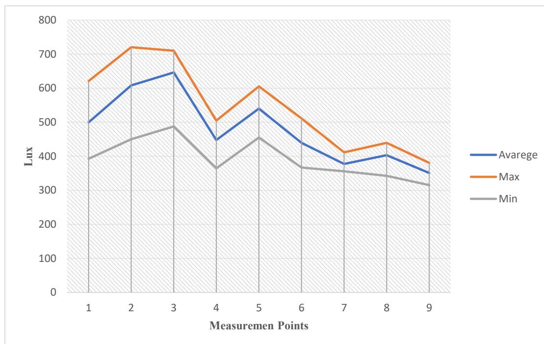
Fig. 9. Measured illumination levels at nine measurement points in the object room.
