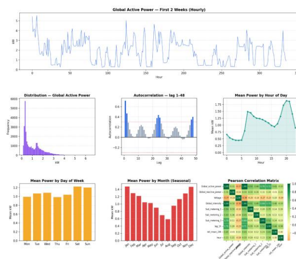
Fig. 2. Exploratory data analysis of the IHEPC hourly dataset: (a) time-series of Global Active Power across the first two weeks; (b) target distribution; (c)
